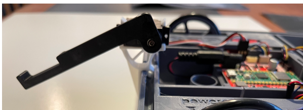
Arm at the other end of rotation positioned behind chassis to pick up objects
